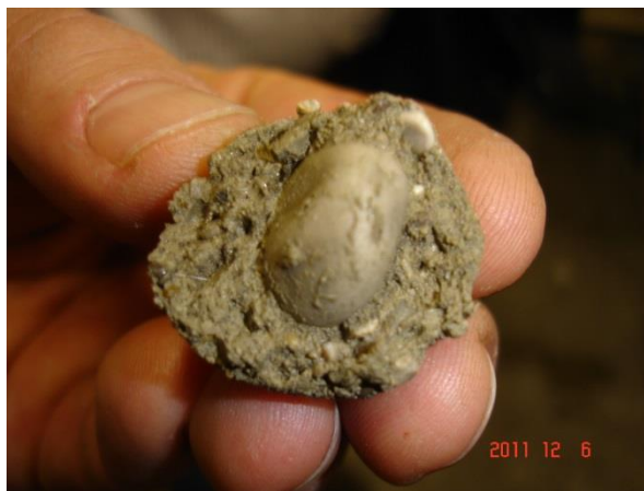
Figure 1. Example of newly formed aggregate from returned concrete
